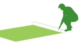
Unroll the grass and position ideally running the pile towards the house on back gardens and the reverse on front lawns (ie facing out). When laying the artificial grass, ensure it fits up to the outer perimeters. Where there is an obstacle like a tree or post fold the grass back and decide the shortest route to cut.
